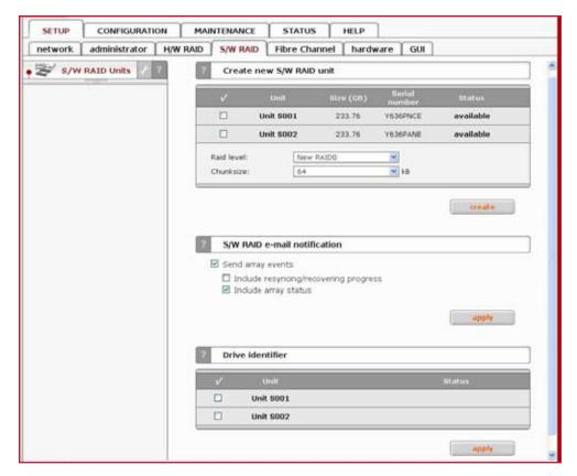
To create a RAID select units, then from ListBox select what type of RAID it will be, then select desired Chunk size. After setting all demanded parameters press Create button.
