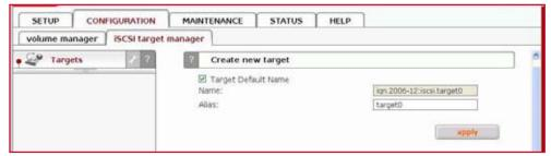
Next in the "Targets" diagram click on the name of a target you have created (e.g. "target0") and within the "Target volume manager" function click the "add" button located by the logical volume in question.
