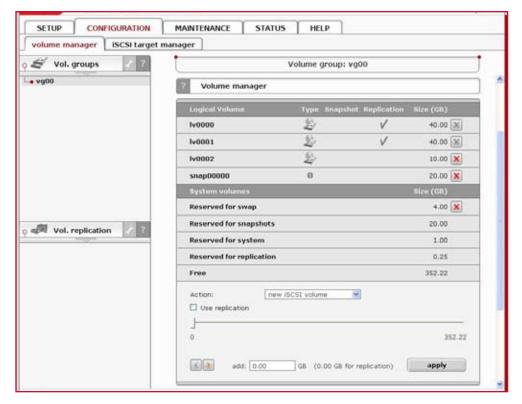
Next, using the "Volume Manager" function you can add disk volume to a new LV, or increase the size of existing LV's (you canot decrease LV size). To set needed LV size just use scrollbar. On the right side of it you will find a counter of available space. This function can be also used to reserve disk space for swap, snapshots, system and replication.
