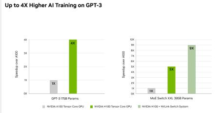
Projected performance subject to change. GPT-3 175B Training A100 cluster: HDR IB network, H100 cluster: NDR IB network | Mixture of Experts (MoE) Training Transformer Switch-XXL variant with 395B parameters on 1T token dataset, A100 cluster: HDR IB network, H100 cluster: NDR IB network with NVLink Switch System Where indicated.
