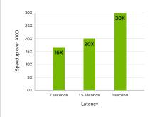
Inference on Megatron 530B parameter model chatbot for input sequence length=128, output sequence length=20, A100 cluster: HDR IB network, H100 cluster: NDR IB network for 16 H100 configurations, 32 A100 vs 16 H100 for 1 and 1.5 sec, 16 A100 vs 8 H100 for 2 sec.
