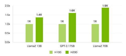
Preliminary measured performance, subject to change. Llama2 13B: ISL 128, OSL 2K | Throughput | H100 1x GPU BS 64 | H200 1x GPU BS 128 GPT-3 175B: ISL 80, OSL 200 | x8 H100 GPUs BS 64 | x8 H200 GPUs BS 128 Llama2 70B: ISL 2K, OSL 128 | Throughput | H100 1x GPU BS 8 | H200 1x GPU BS 32.
