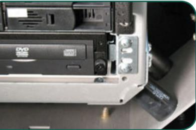
Shock absorbers line the chassis, keeping the system protected from sudden impact as well as sustained vibration.
