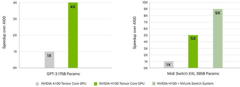
Projected performance subject to change. GPT-3 175B Training A100 cluster: HDR IB network, H100 cluster: NDR IB network | Mixture of Experts (MoE) Training Transformer Switch-XXL variant with 395B parameters on 1T token dataset, A100 cluster: HDR IB network, H100 cluster: NDR IB network with NVLink Switch System where indicated.
